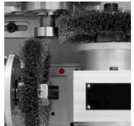
Twin deburring station
