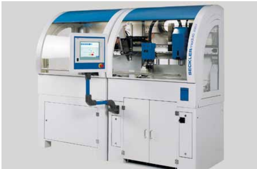
Twin cell: extending by interlinking more than one modulo cell
