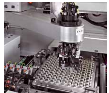
SCARA arm with double gripper
