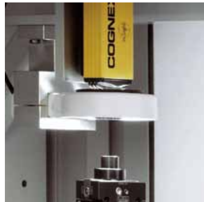
Orienting station with camera
