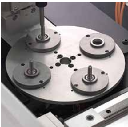
Rotary indexing bench with measuring station
