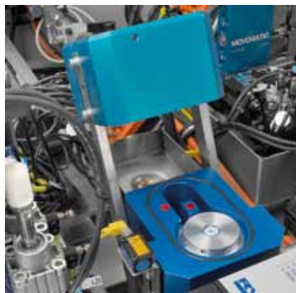
Station de lavage
