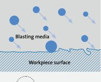
Compression of the surface with simultaneous embedded additives inside the surface. Increase of the tribological characteristics for various applications.
