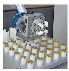
The robot is loading and unloading the rotary table of the micro sandblasting system.
